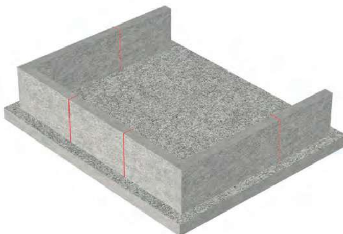
Cracks created using ERFLEX BV
