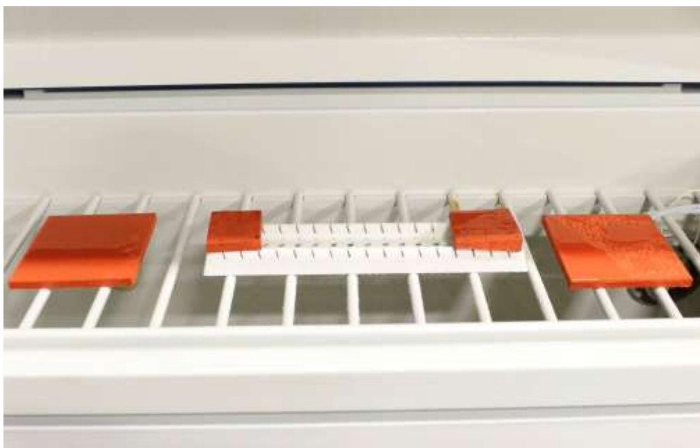
Picture 1. Arrangement of specimens in the spray cabinet.
