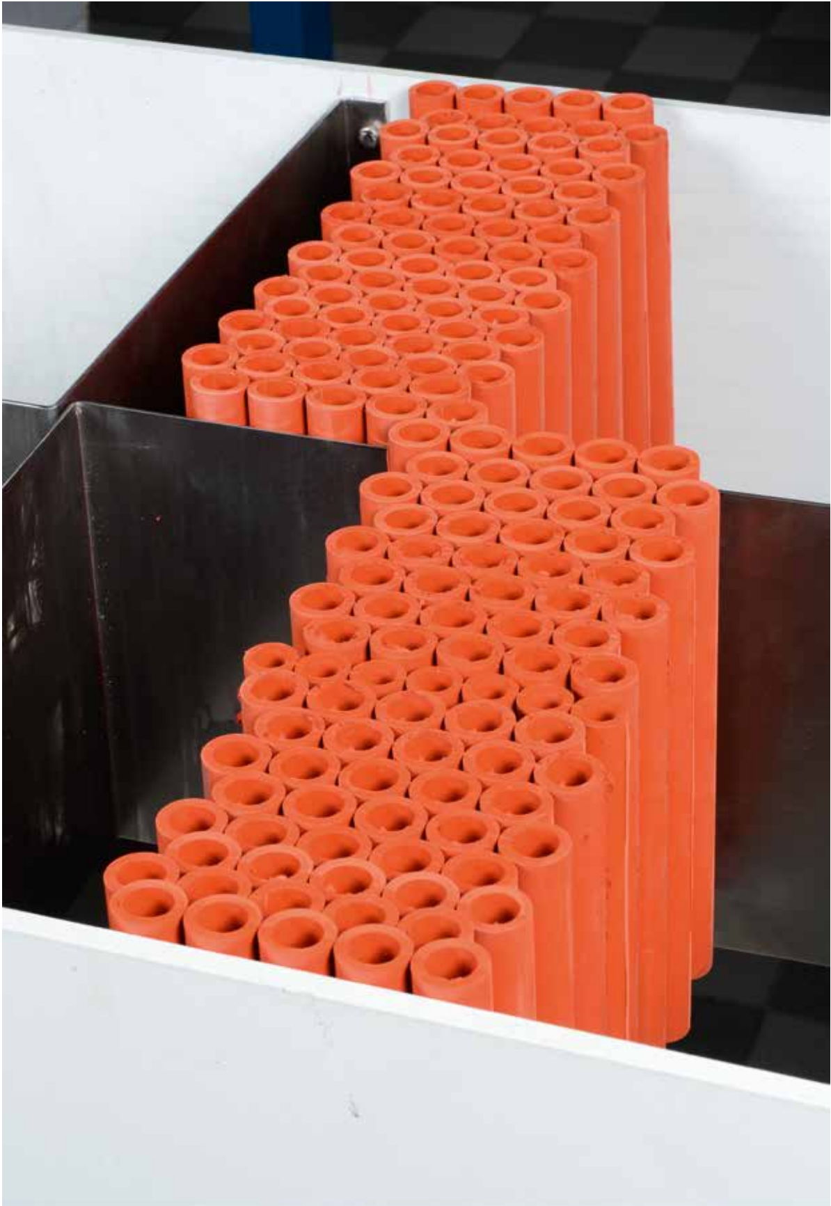
The stacked sets of filler sleeves placed at both sides of the partitions. At this stage the position of the filler sleeves is not important.
