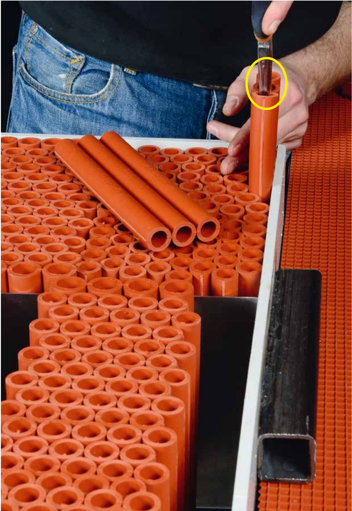
The flexibility and the smooth surfaces of the filler sleeves make insertion of the smaller sets of filler sleeves or single sleeves easy when using a flat nose pliers.
