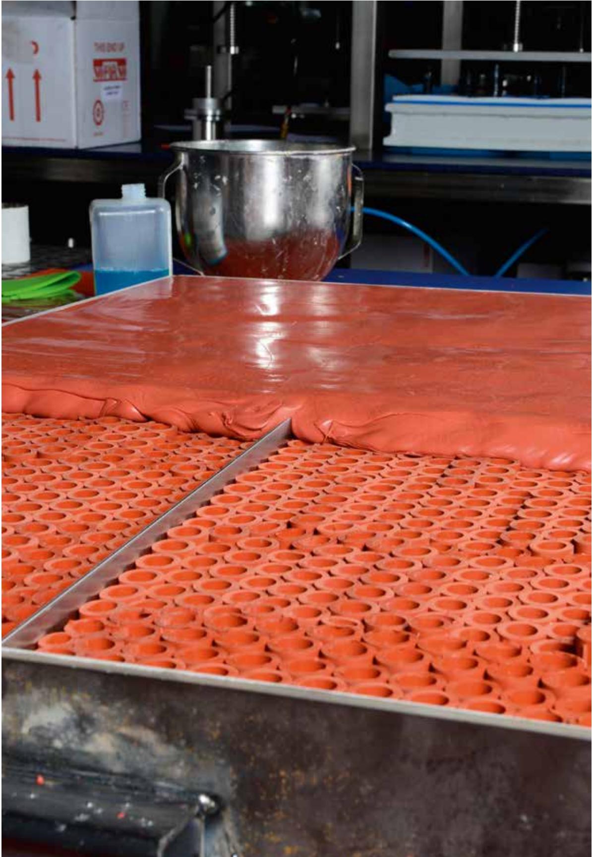
View on the finished and non-finished part of the NOFIRNO gap seal.
