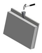
Adhesion to the formwork should be minimised before lifting the concrete element out of the formwork by removing as many parts of the formwork as possible.
