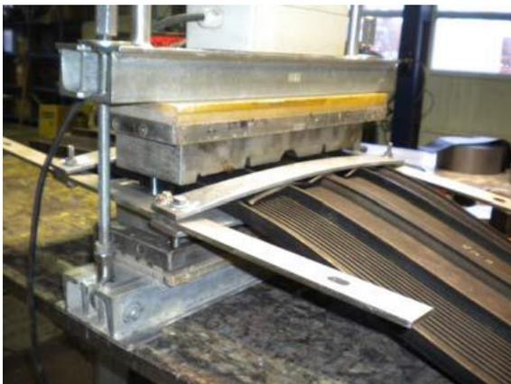
\*) In strong wind and at low outside temperatures, the vulcanization unit should be covered up with foils and formwork panels. At temperatures around the freezing point, vulcanization is only possible with a very great deal of effort, such as the construction of a boarding and heating with fan heaters. However, this is hardly feasible in practice and therefore we recommend not to vulcanize at these temperatures.
