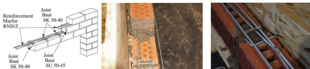
Fig. 2. A structural solution of brick lintels.
