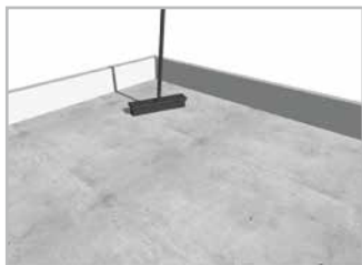
Preparation of a base according to DIN 1045-2 Compacted, clean planum. Concrete subbase according to DIN EN 206-1 and DIN 1045-2.
