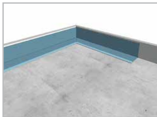
Fitting and securing of the manually prepared Polyfleece SX ® 1000-stripe along the side formwork (width of stripe depending on height of side formwork PLUS 10 cm horizontal overlap). The horizontal overlap must be at least 10 cm.
