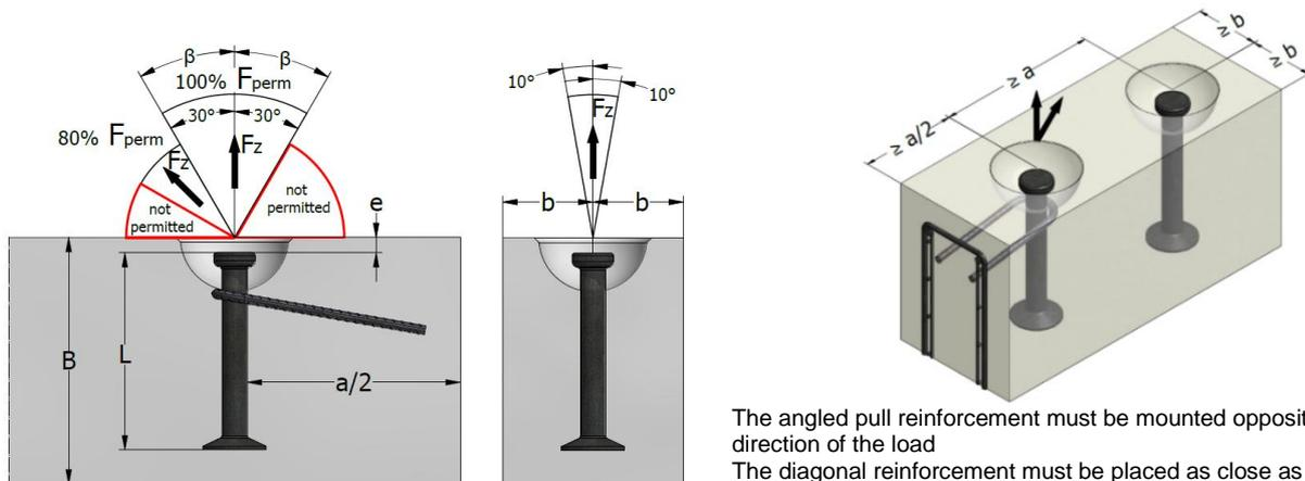
The angled pull reinforcement must be mounted opposite the direction of the load
