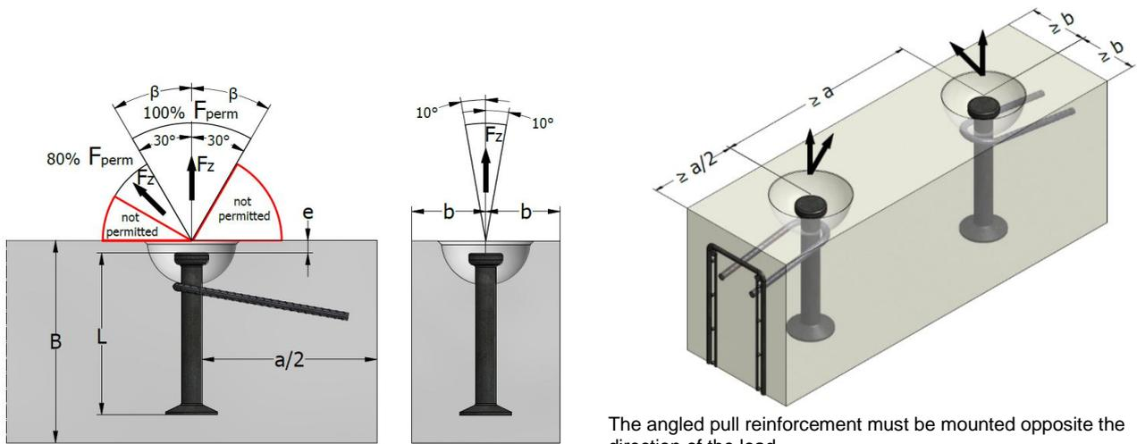
The angled pull reinforcement must be mounted opposite the direction of the load
