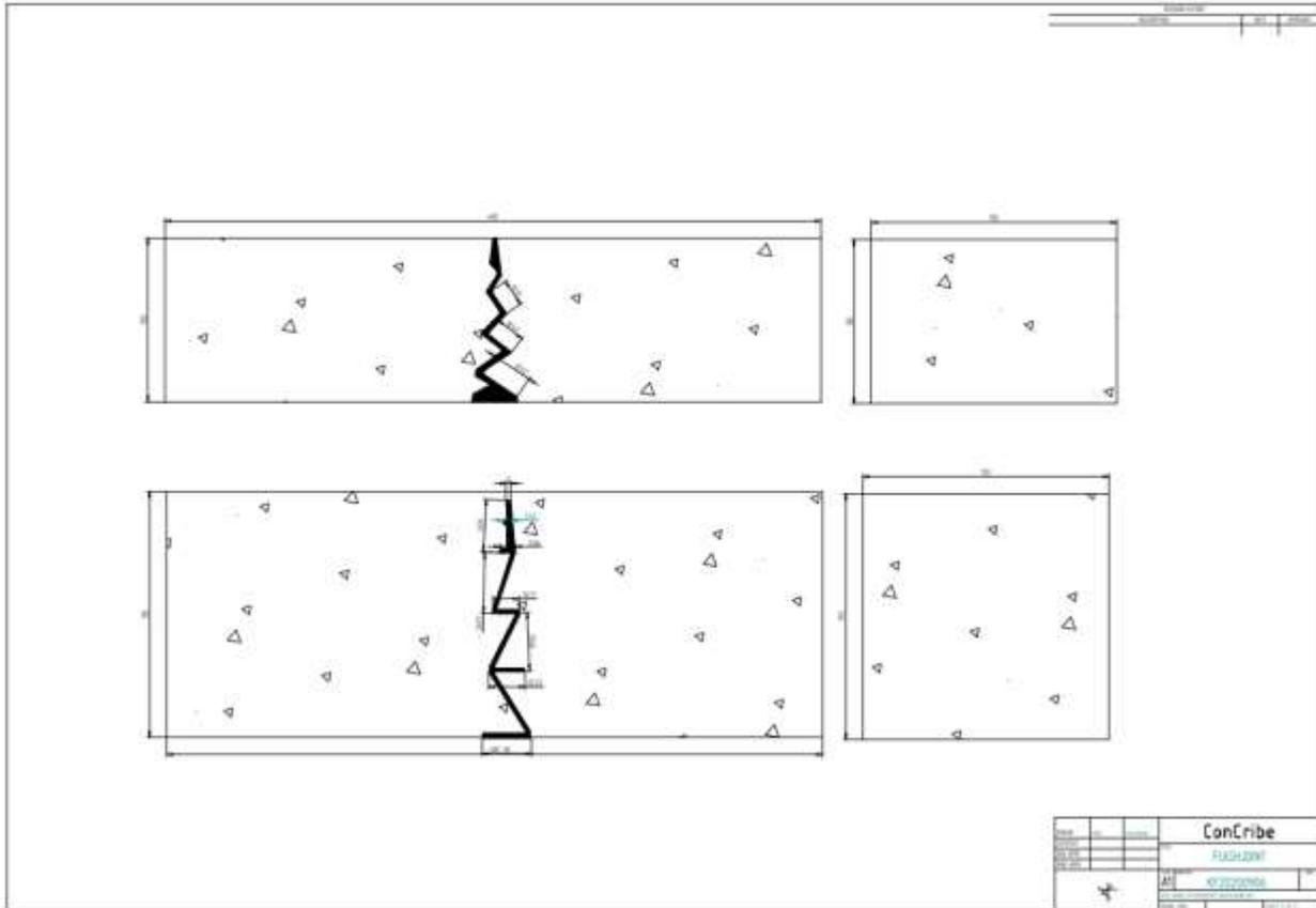
Design of the test beams and location of the flashjoint 100 and 150.
