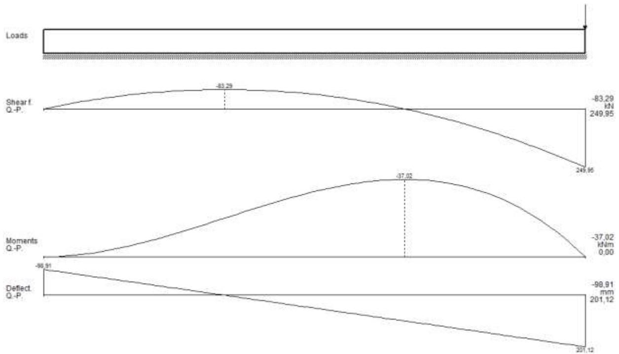
Shear force in the joint : 250 kN/m
