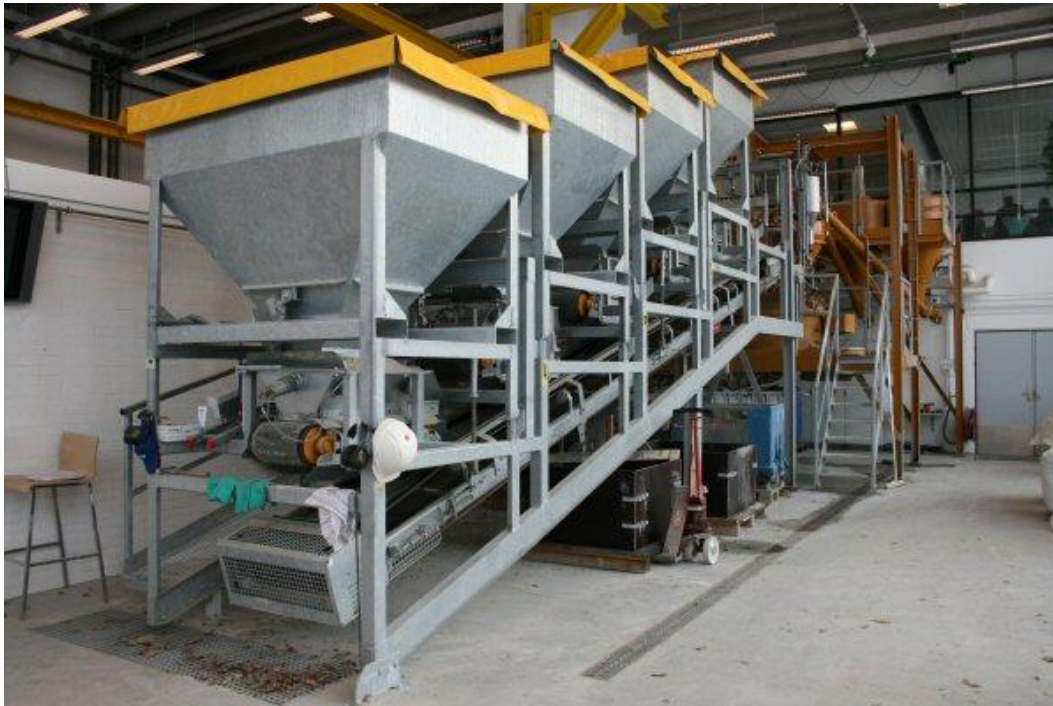
Photo 1: The mixing station is equipped with a 375/250 liter counter-current mixer, five aggregate silos and four powder silos from Haarup A/S, and process control software from Skako A/S.
