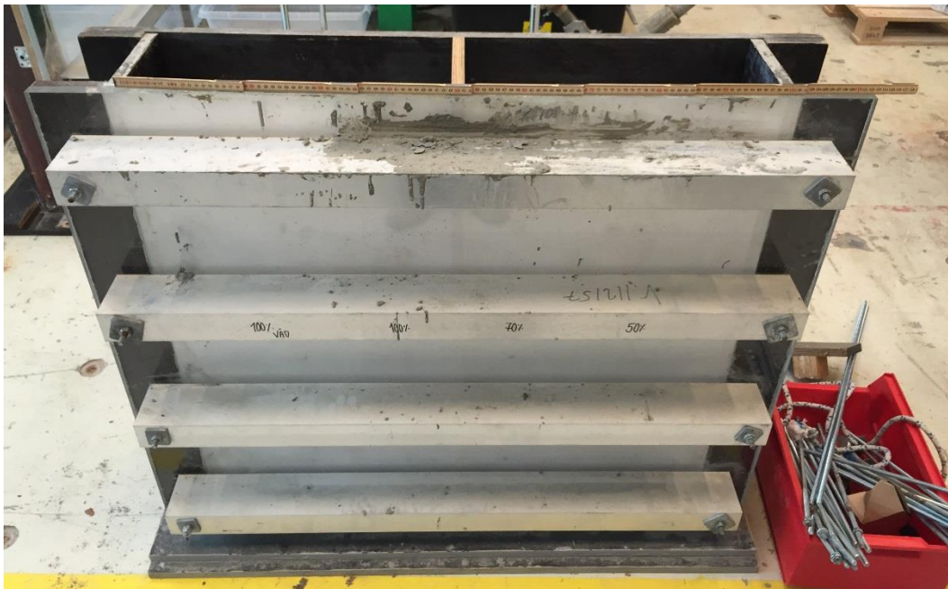
Photo 2: The formwork for the two concrete blocks has plywood on one side and CPF liner on the other side (seen through plexiglass in photo). The two blocks were cast from the same batch and separated by a plywood plate in the middle of the mould.
