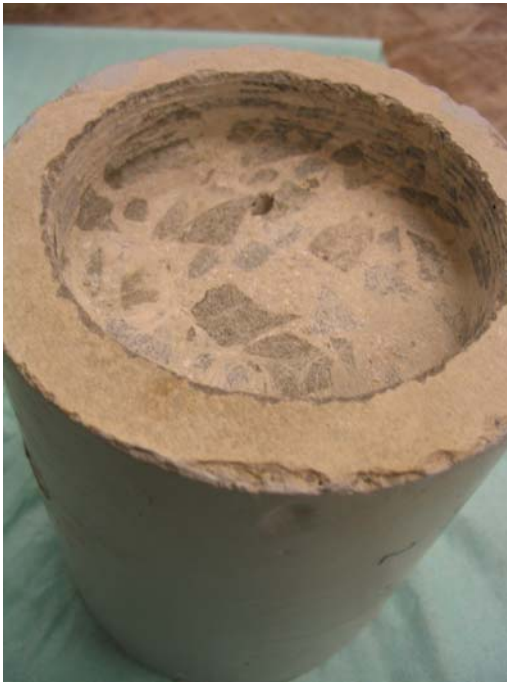
Fig. 10 Core after dust samples were removed.
