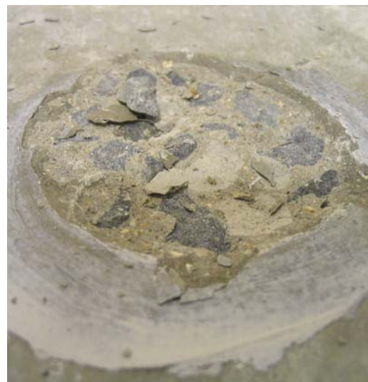
Fig. 6b Concrete surface after a pull-off test
