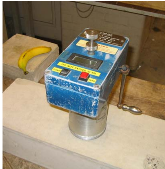
Fig. 5b Limpet Pull-off Tester
