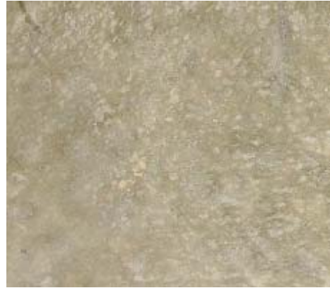
Fig. 14 Concrete cast using Formtex CPF
