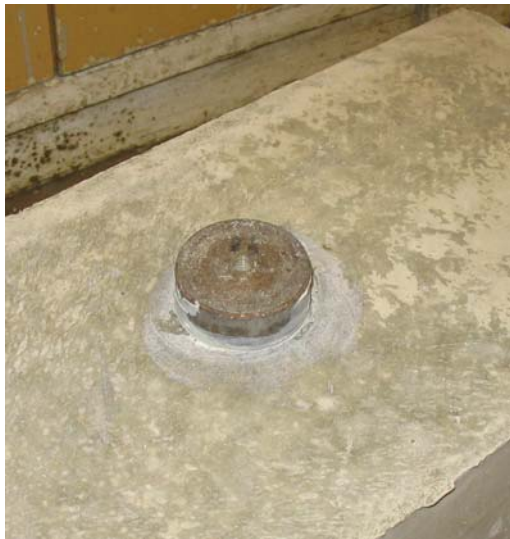
Fig. 5a Pull-off probe
