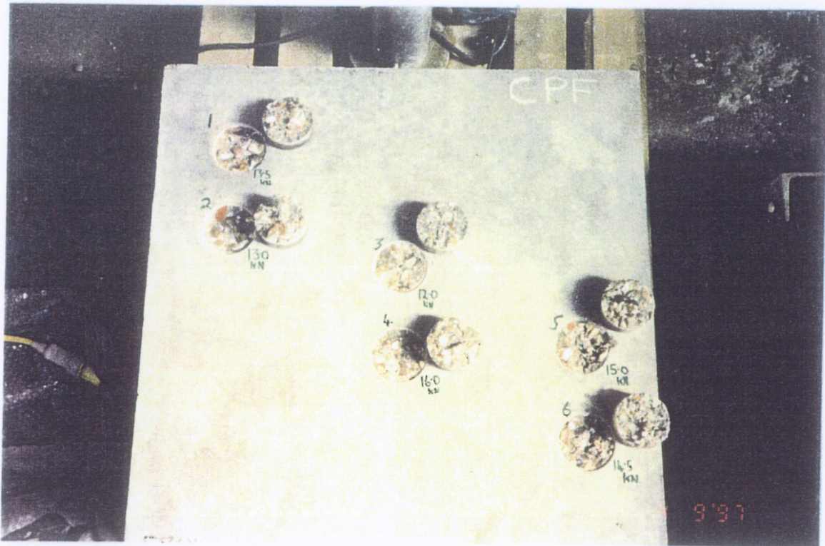
BOND-TEST: CPF FACE OF PANEL AFTER TESTING
