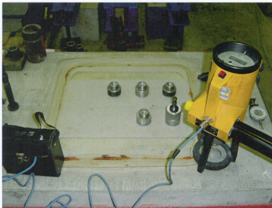
Fig. 7: Testing the tear-off resistance after the coating was exposed to pressurised water for 4 months
