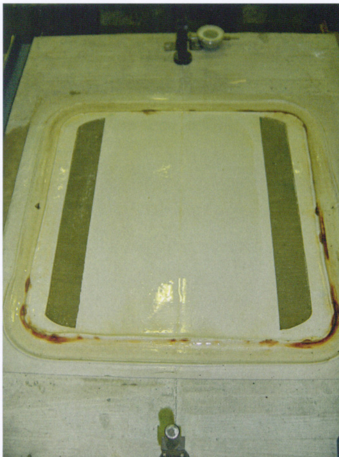
Fig. 6: Disassembled test specimen after the sealing test with the marking of the joint under the coating
