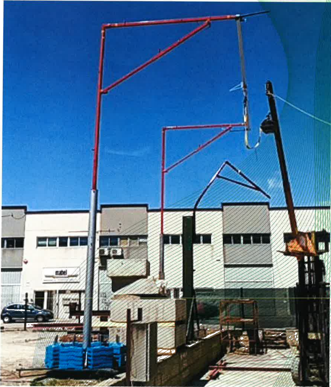
Fig. 4: Anchor device type D (type Horizontal SafeAccess and NAV2 trolley made by FALLPROTEC SA) with anchors of type AlsiPercha and mobile base units
